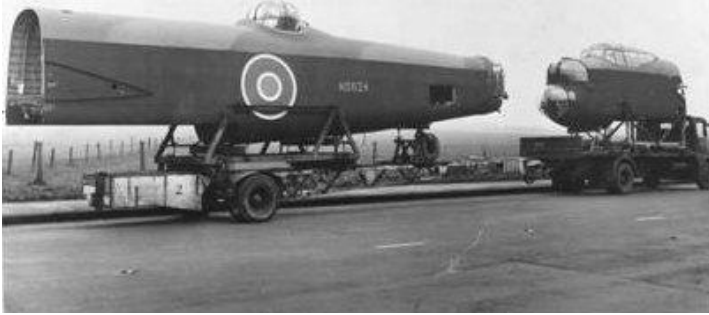
Fresh from the factory, ND924 leaves the Avro facility at Chadderton for final assembly at Woodford.
