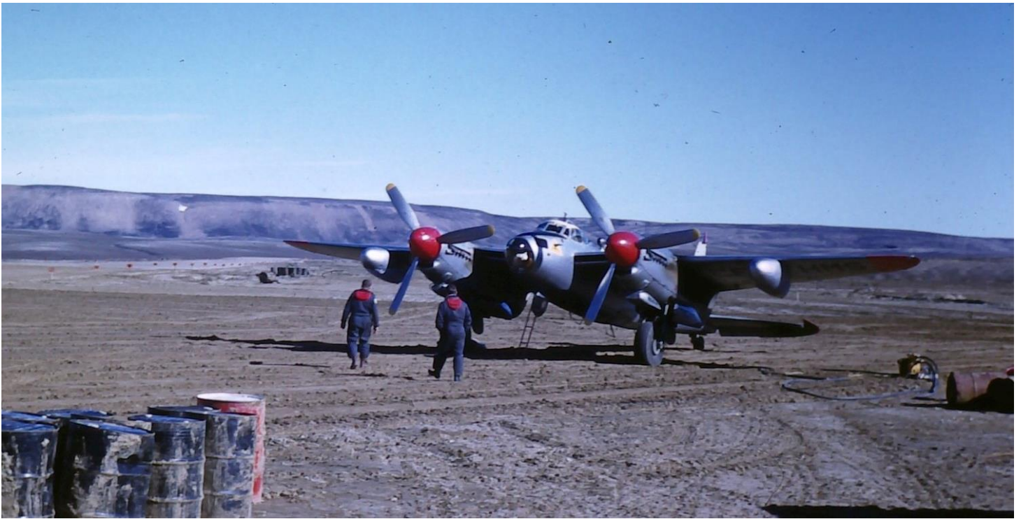
Canadian-built de Havilland DH.98 Mosquito operating from a remote and rough airstrip which Spartan had built at Pelly Lake, Northwest Territories (Now Nunavut) in 1958. Spartan's work with Mosquitos in the far North faced extreme logistical challenges for fuel, maintenance and weather information. Photo via the Author
