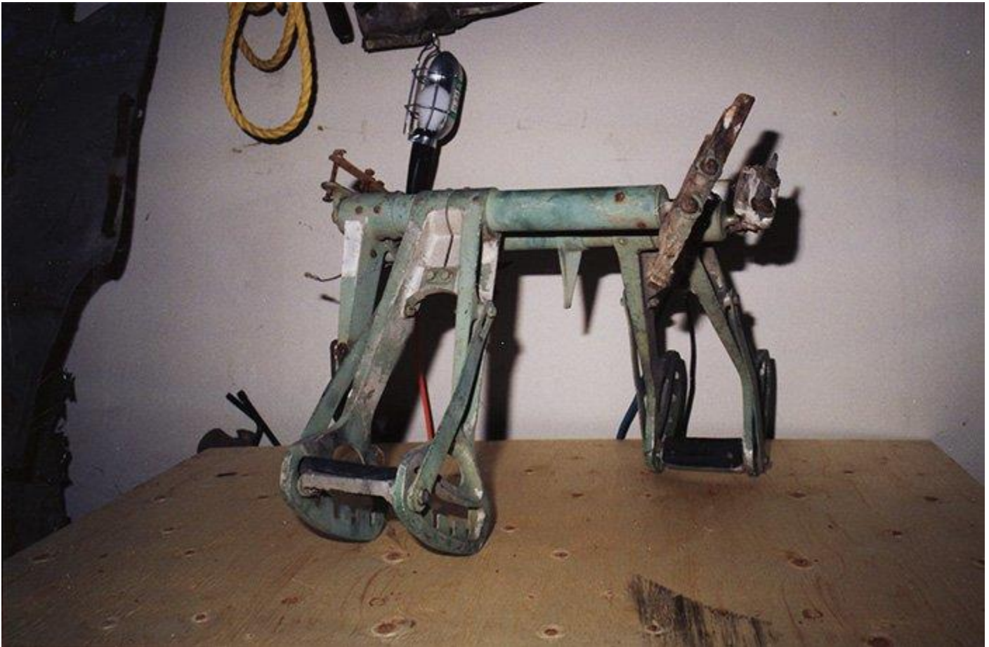
A pair of Canadian-built de Havilland Mosquito main wheels (top) and rudder pedals. All had been kept indoors since being removed from KA114 and showed no overt signs of corrosion. Photo: Richard de Boer
