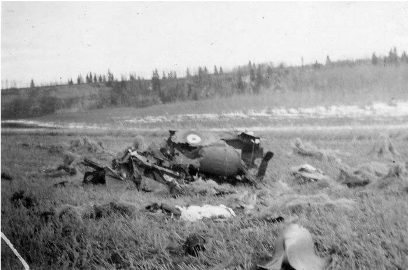
A rather catastrophic crash of an Airspeed Oxford at Penhold. The scalloped metal piece at the bottom right is the upper trailing end of the engine nacelle. Photo via Robert Barnes Collection
