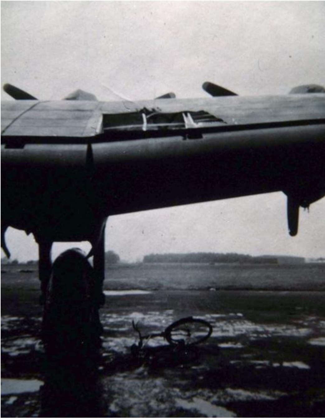
Damage caused to Halifax NP692 main wing, almost reaching the fuel tanks. [Doug Penny]
