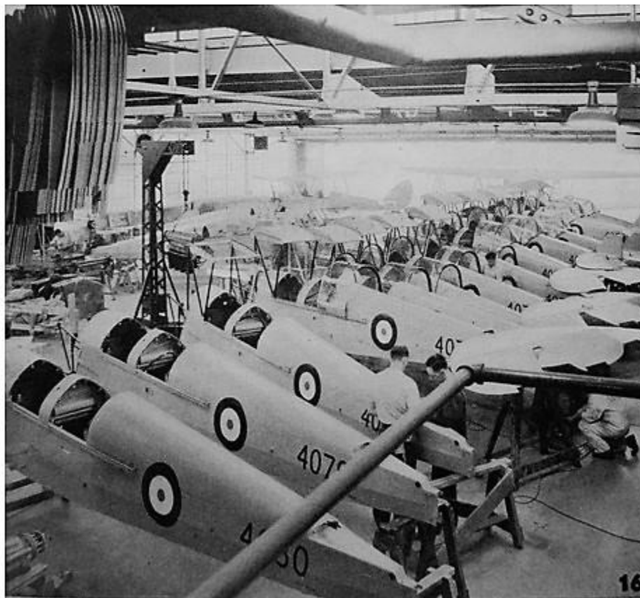
16. Step by step the machine goes down the fuselage assembly line. Hundreds of Canadian pilot fledglings will first take to the air in craft like these.
