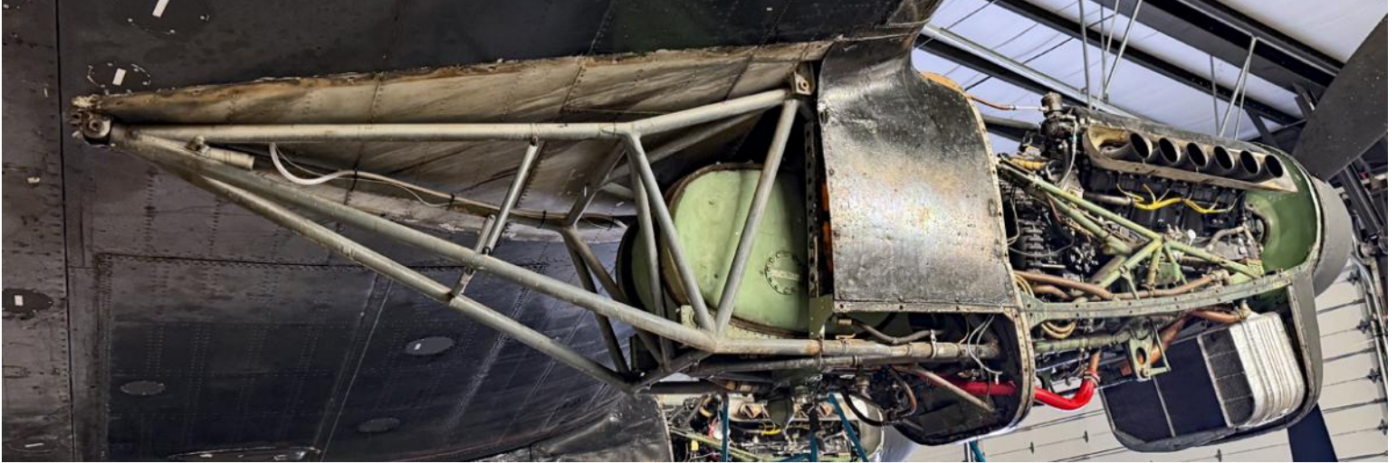
The starboard-outer Merlin with the nacelle and cowls removed.
