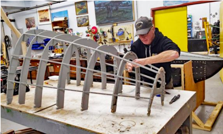
Brian assembling the components of the nacelle framework. Much of the original frame had completely rotted away. Apparently there's much more wood in a Lancaster than one would expect. Note the nacelle skin to Brian's left.
