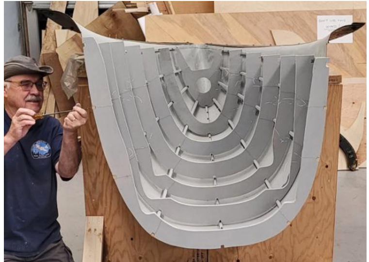
Gary from the Mosquito group helping to test-fit the framework to the metal nacelle skin.
