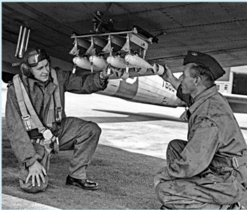
Prior to a flight at a Bombing and Gunnery School, a student bomb aimer inspects practice bombs attached below the wing of a Fairchild. When the bomb struck the ground, it emitted coloured smoke. As there was more than one bomb aimer in the aircraft, observers on the ground used the different colours of smoke to determine the accuracy and the identity of each bomb aimer.
