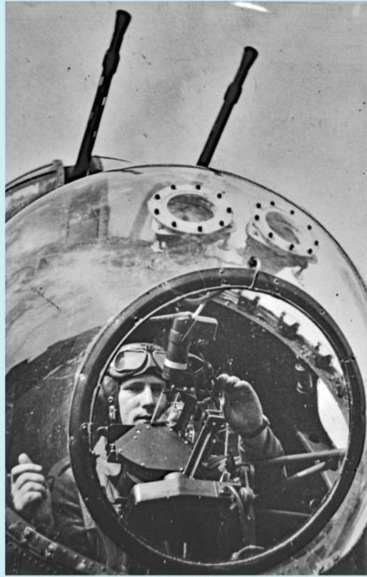
A bomb aimer looks through his bomb sight in the nose of a Lancaster bomber. His right thumb is on the release button.
