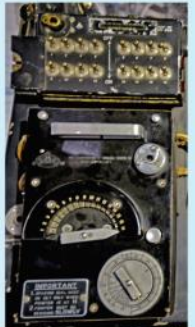
The bomb aimer's control panel enabled him to release bombs from up to sixteen different locations in the bomb-bay.
