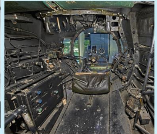
Looking into the bomb aimer compartment in the nose of a Lancaster. Note the 'computer' (at left), the bomb sight (centre) with the chest cushion below, the bomb aimer's panel (to the right of the cushion), and the mesh container for a portable oxygen bottle (at right).
