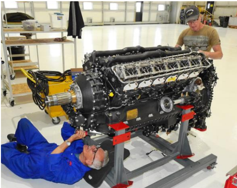
CMS Board member Dick Snider and Merlin/Lanc man from the Bomber Command Museum, Brian Taylor put the finishing touches on the timing for the Hurricane's Merlin 29 engine.
