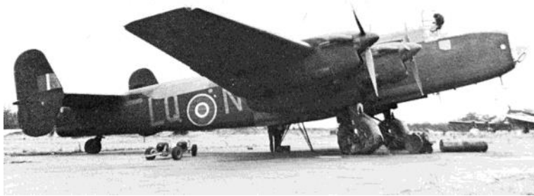
405 Squadron Halifax -The container under the nose is an overload fuel tank, fitted in the bomb-bay for long flights such as those to Berlin.
