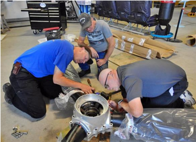
Following inspection and servicing, the propeller for the Lancaster's starboard-outer engine was reassembled and placed on the aircraft.
