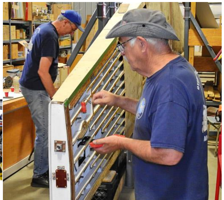
A significant moment as Gary T. rolls glue on the stringers of the starboard upper wing surface just prior to installing the first new skin. It's been two years since we jiggered the wing and began stripping and cleaning it as well as a year to source the proper spec plywood.
