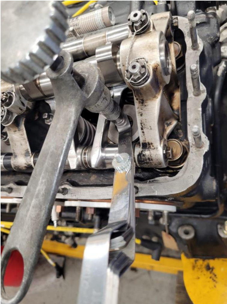
Special Merlin tool for setting clearance
