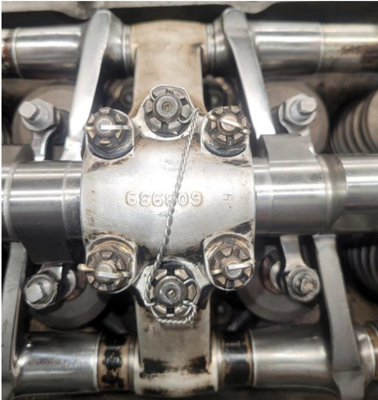
Cam supports lock wired and cotter pinned
