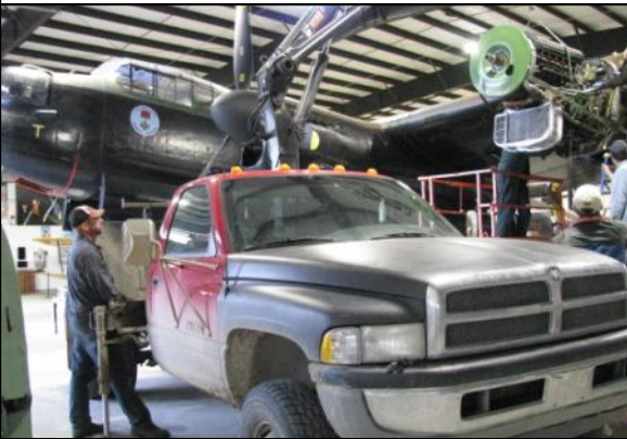
Ben Schwartz operates his picker-truck to lift the Merlin for reinstallation on the Lanc.
