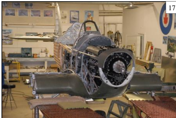
The CMS Hurricane's fuselage seen here in an advanced stage of being restored.
