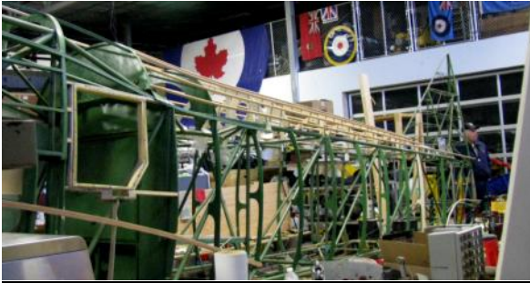
The fuselage turtle-deck frame stringers all in place. Some previously built fuselage formers had to be redesigned and replaced.
