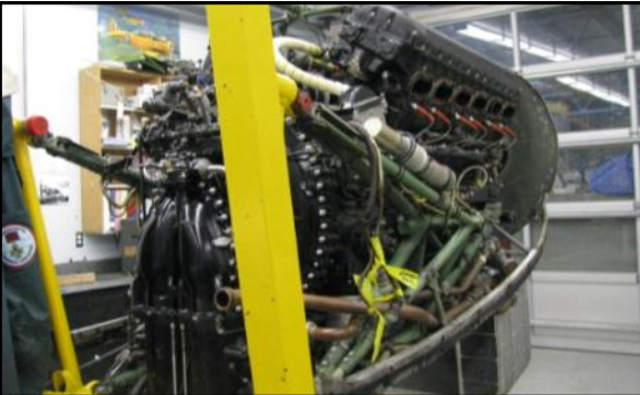
Merlin #1 reassembled ready to reinstall.
