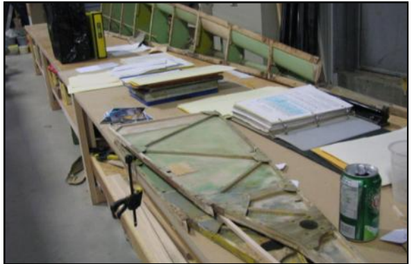
In the trailing wing edge in the background. In front one of its ribs being rebuilt.
