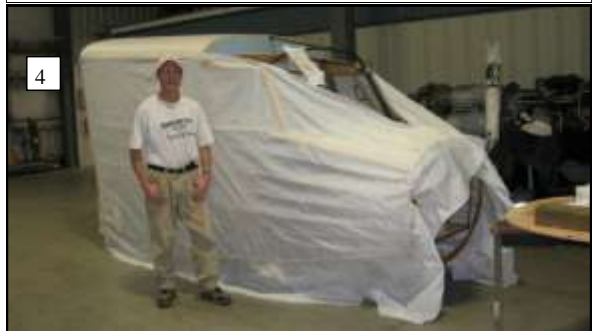
(4)Kevin Charlton standing on the starboard side of the Cessna Crane cabin section to which the Polyfabric is attached and ready to be trimmed and shrink-tightened with a seamstress' iron in his steady hand.
