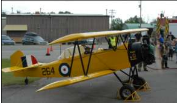
The museum's restored Fleet Fawn, bi-wing, training airplane which was used to train pilots during WWII. Here its Kinner engine is being run-up.
