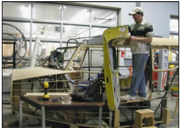
Kevin Charlton seen here working on the Cessna Crane cabin section that is being made into a "flight Simulator". Kevin is a different kind of craftsman; he makes and repairs guitars. His skills can be seen in the woodwork he is doing on the Crane. See page 6 for more about this project.
