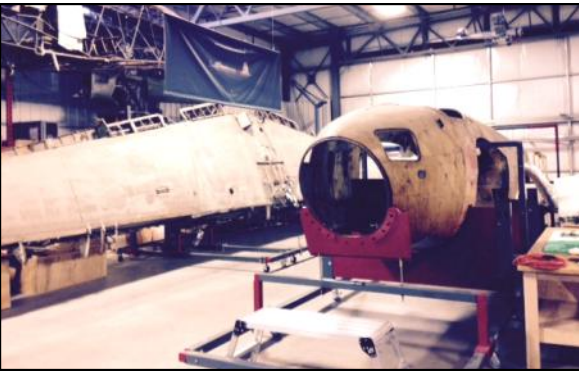
The Mosquito on new rolling stands along with fuselage on its construction stand.
