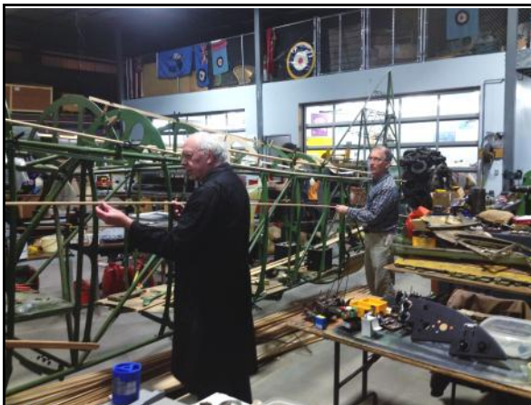
Carl Orde and Terry Moynihan shown here trial fitting the fuselage stringers.
