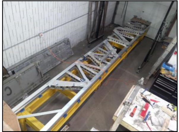
New main spar on 30 foot jig table - note rear spars of center section on wall to be rebuilt next.
