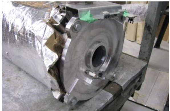
The removable end of a new exchanger. A much easier and should be less expensive repair than replacing the whole exchanger. Learned at customers expense?
