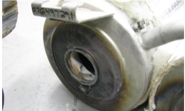
Photo shows end of an original heat exchanger. Looking close just inside the opening you can see a gouge where a piece of the ceramic has broken away. All three exchangers had similar damage.
