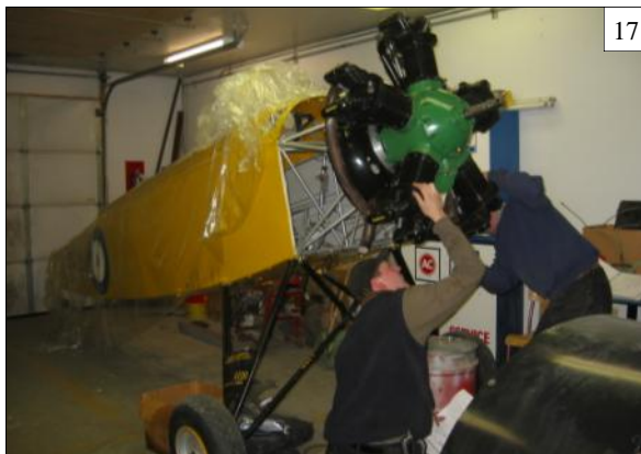
Greg Morrison and Gordon Neu fitting the Kinner engine to the Fleet Fawn (lean-to shop.)
