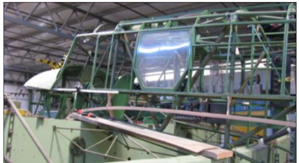
Photo shows one of the Anson's restored windows mounted in the fuselage.
