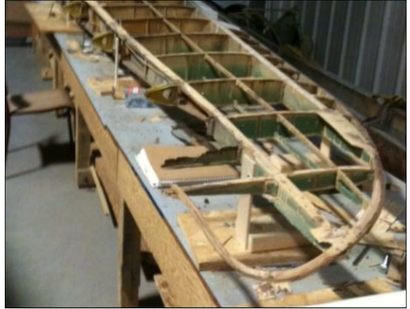
The horizontal stabilizer (tail plane) is being restored - note the restored ribs.
