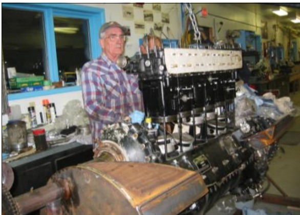
Rebuilding the first Merlin engine in the lean-to shop, John Phillips standing - two more engine crew out of sight behind.
