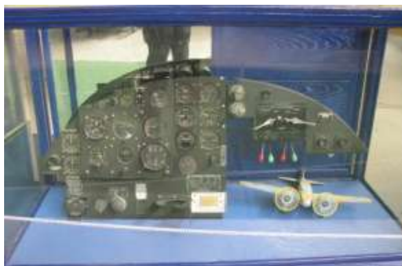
Avro Anson Mk. II mail panel is shown with a model of the aircraft.
