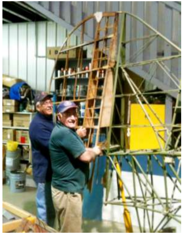
Wayne Bailey and John Maze trial fit the Anson rudder that John has been restoring. (80% of the original wood used.)
