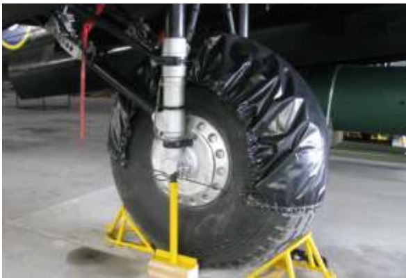
New oil resistant tyre covers have been made for the Lancaster's main gear.
