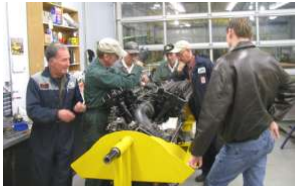
The "engine crew" is in the final stages of reassembling the Lanc's, in-board Port Merlin engine.
