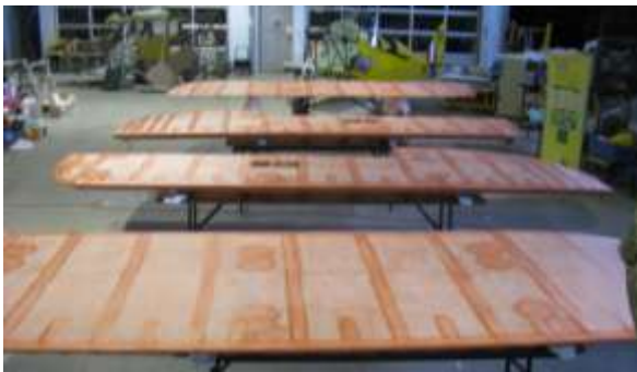
The Tiger wings are covered and await the final coats of paint.
