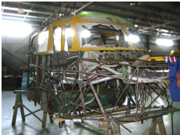
This Cessna Crane forward fuselage is being converted and restored for use as the body of a second flight simulator for the museum.
