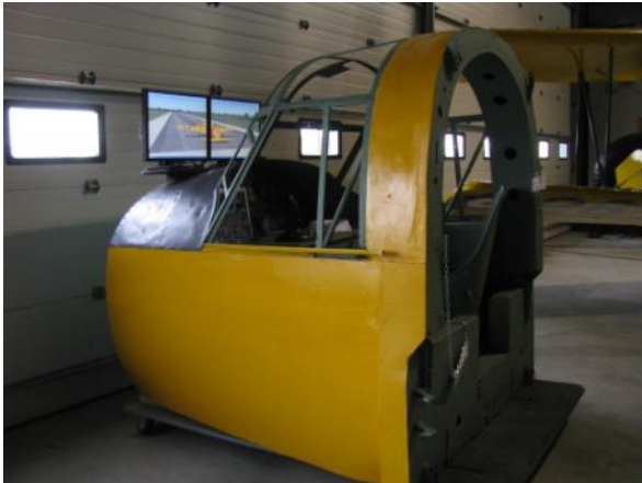
These three photos show the stages of condition of the Mk.V Anson cabin section as it was converted into a flight simulator body as a “hands-on” display for use by visitors to the museum.
