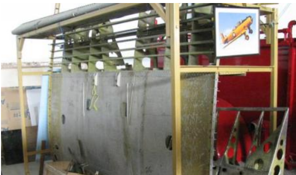
Yale centre section awaiting a new spar.
