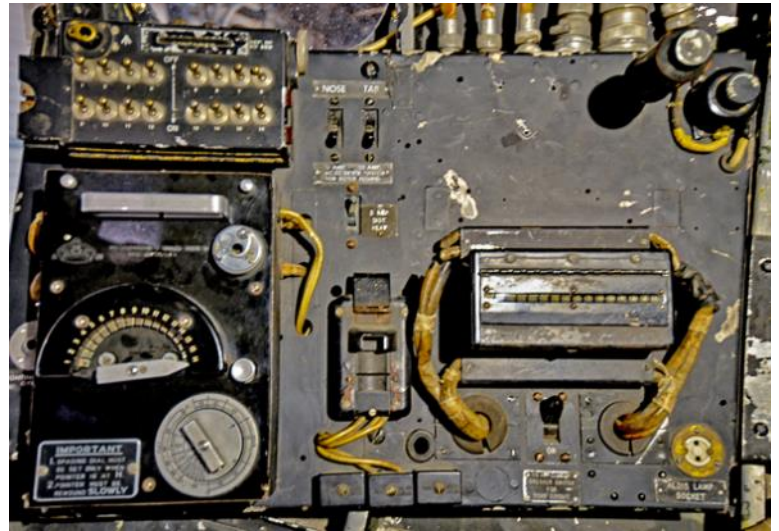
The bomb aimer's control panel enabled him to release bombs from up to sixteen different locations in a Lancaster's bomb-bay.
