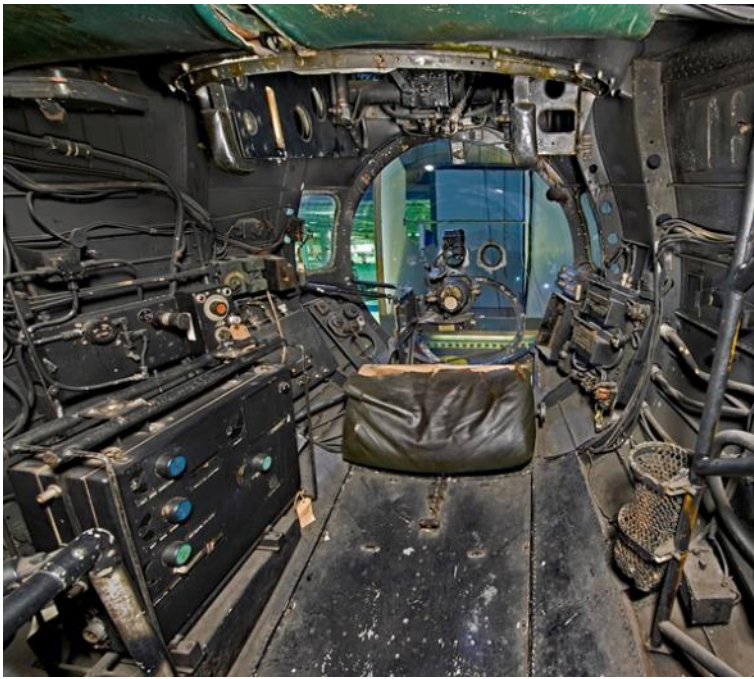
Looking into the bomb aimer compartment in the nose of a Lancaster. Note the 'computer' (at left), the bomb sight (centre) with the chest cushion below, the bomb aimer's panel (to the right of the cushion), and the mesh container for a portable oxygen bottle (at right).
