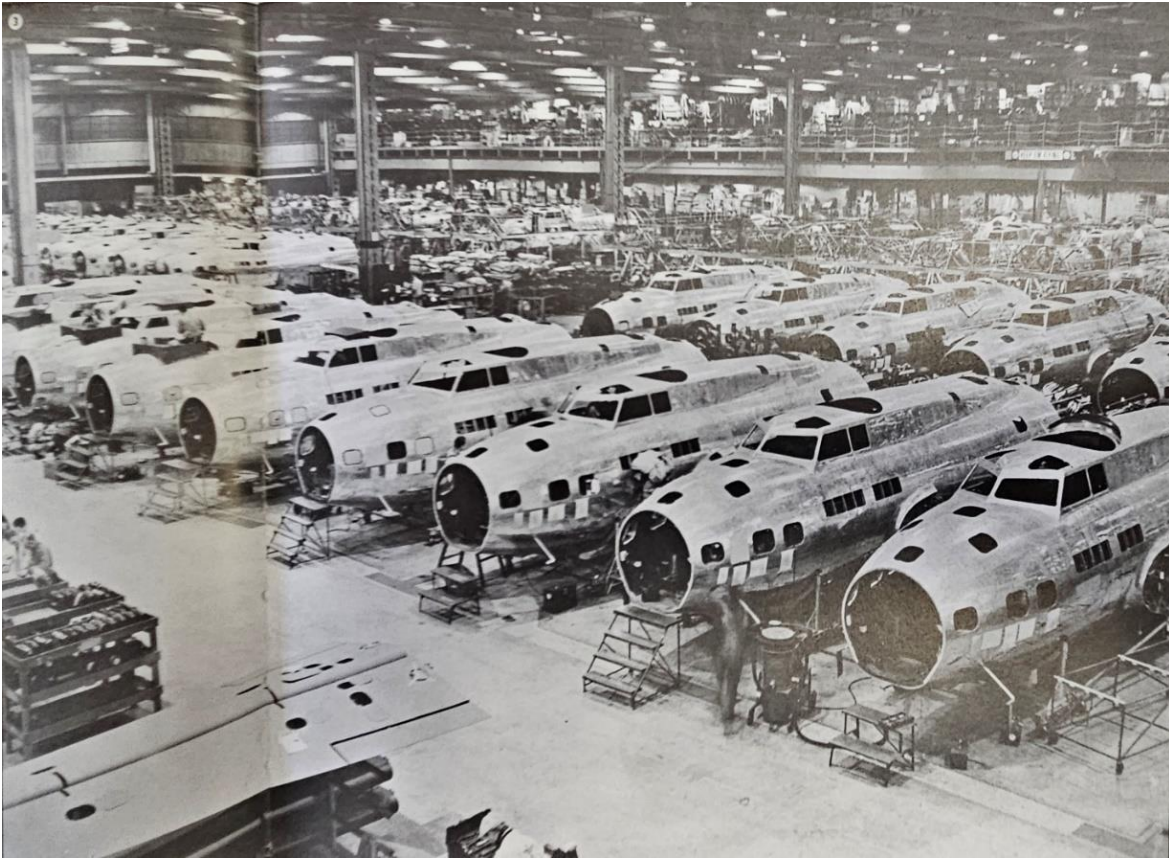
B-17 MAIN BODY ASSEMBLY LINE AT BOEING FACTORY IN SEATTLE. (Source - B-17 Flying Fortress )
